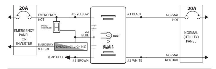
**Wiring Diagram #2:** Slave Relay Application - RRU-UNV can be used to switch an auxiliary load (similar to a lighting contactor) in case your switch is rated <20A or to switch a 277V load from a 120V switch.
