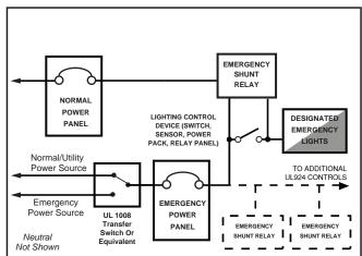
**Wiring Diagram #1:** A dedicated switch or line voltage dimmer controls emergency lighting in a space. Upon loss of normal power, the emergency lighting comes on at full brightness regardless of switch or dimmer position. NOTE: RRU-UNV is not for use with 0-10V DIMMER. Use RRU-X-UNV or EPC-2-D.
