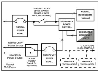
**Wiring Diagram #1 (Suggested):** A common switch controls both normal and emergency lighting in a space. Upon loss of normal power, the emergency lighting comes on regardless of switch position.
