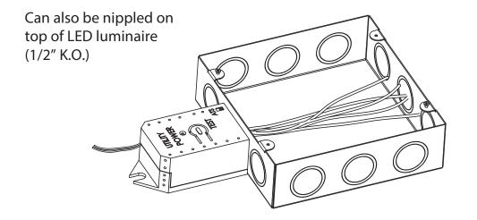
Tested to UL2043, Plenum Rated
