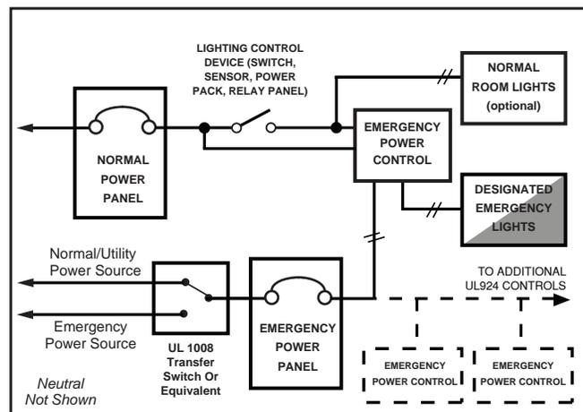
**Wiring Diagram #1 (Suggested):** A common switch controls both normal and emergency lighting in a space. Upon loss of normal power, the emergency lighting comes on regardless of switch position.
