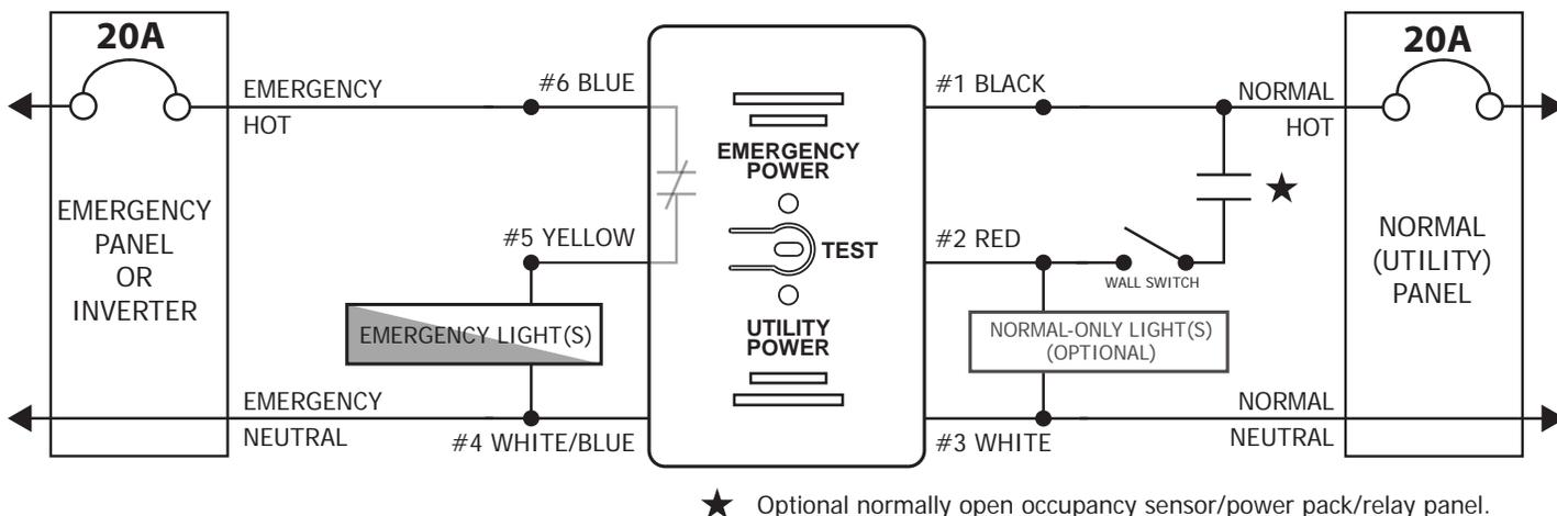
**Wiring Diagram #2 (Shunt):** A dedicated switch controls emergency lighting in a space. Upon loss of normal power, the emergency lighting comes on regardless of switch position.
