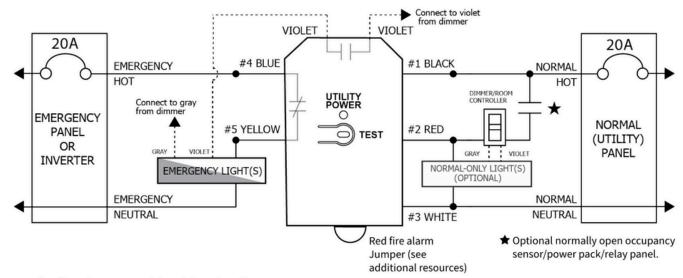
Contact factory for fire alarm override wiring detail.
