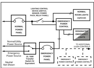
**Wiring Diagram #1 (Suggested):** A common dimmer controls both normal and emergency lighting in a space. Upon loss of normal power, the emergency lighting comes on at full brightness regardless of dimmer position.
